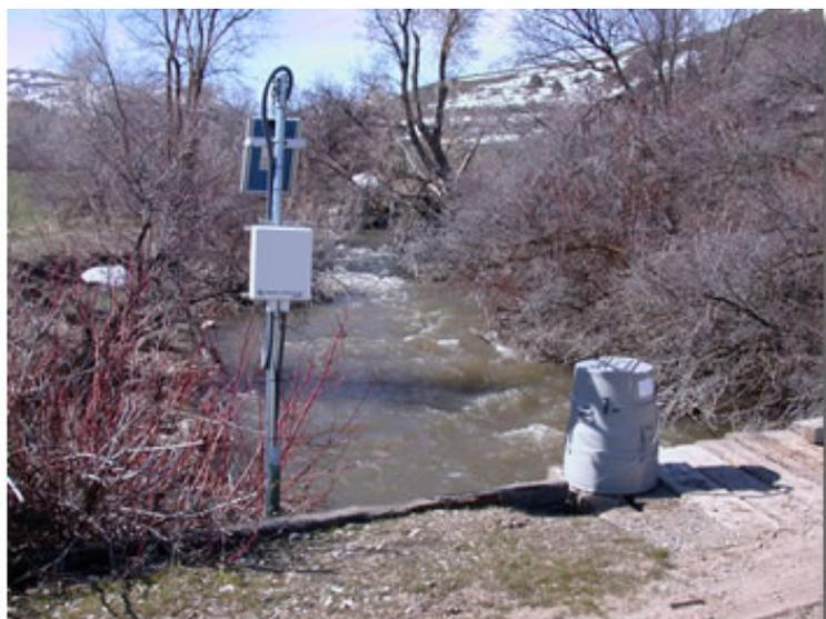
*Continuous measurements in the Little Bear River are combined with lower-frequency automated and grab samples to create high-frequency estimates of water quality constituent concentrations.*
